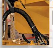
Pig's Tail™ protective wrapping is manufactured to the highest standards. By only using "virgin grade" high density polyethylene, our products exhibit superior wear resistance and extremely good environmental stress crack resistance (ERS).
