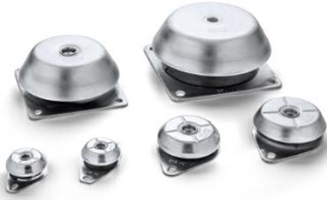
AMC Mecanocaucho® BRB Captive anti vibration mounts are anti vibration elements which work the rubber in shear and compression. Their high profile rubber sections produce larger deflections, low natural frequencies. This range of mounts is suitable for applications where vibration isolation is a priority.
