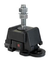
The AMC Mecanocaucho® MARINE XT Captive anti vibration mounts are anti vibration elements which work the rubber in both shear and compression. Their design has been tailored to provide a specific stiffness in each axis, a key benefit is providing a reduced roll natural frequency for engine installations.
